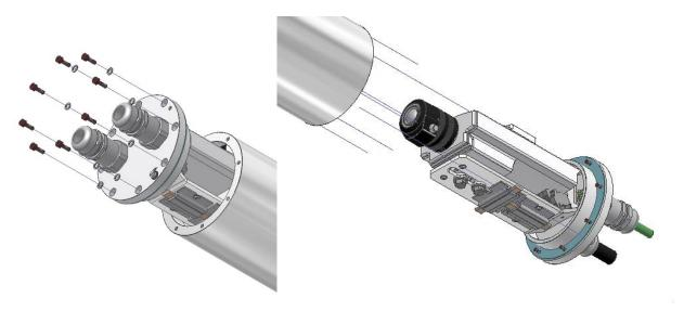
Figure 6-2 Opening the RoughCam IPM2036 (similar illustration)
