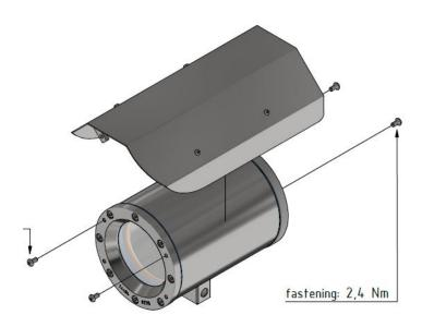
Figure 6-1 Removing the weather protection roof
