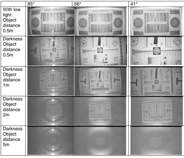
In absolute darkness, the internal infrared illumination can only be used up to a maximum object distance of 2.0 m. In addition, the quality of the image is strongly influenced by the resulting reflections and the object to be observed is no longer visible.
