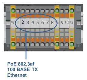
Figure 5.7 – Connection to the terminal box
