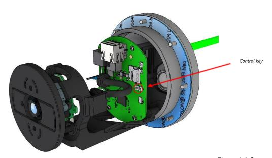
Figure 6-3 Structure of the camera
