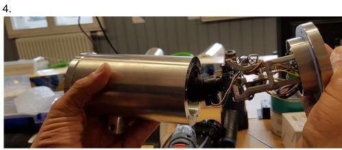
Figure 5.3 removing the camera
