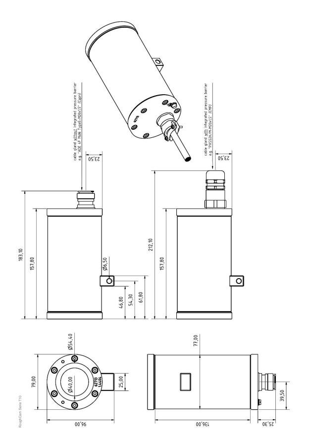
Figure 10.1 – Dimensions of the T10 RoughCam e.Vario
