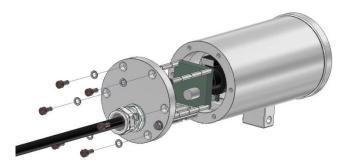
Figure 5.2 – Opening the RoughCam e.Vario
