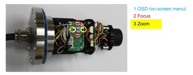
Figure 5.1 - RoughCam® e.Vario - Lens and sensor board
