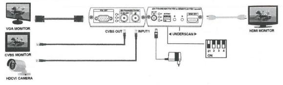
Figure.5.6 - Signal-output-variants
