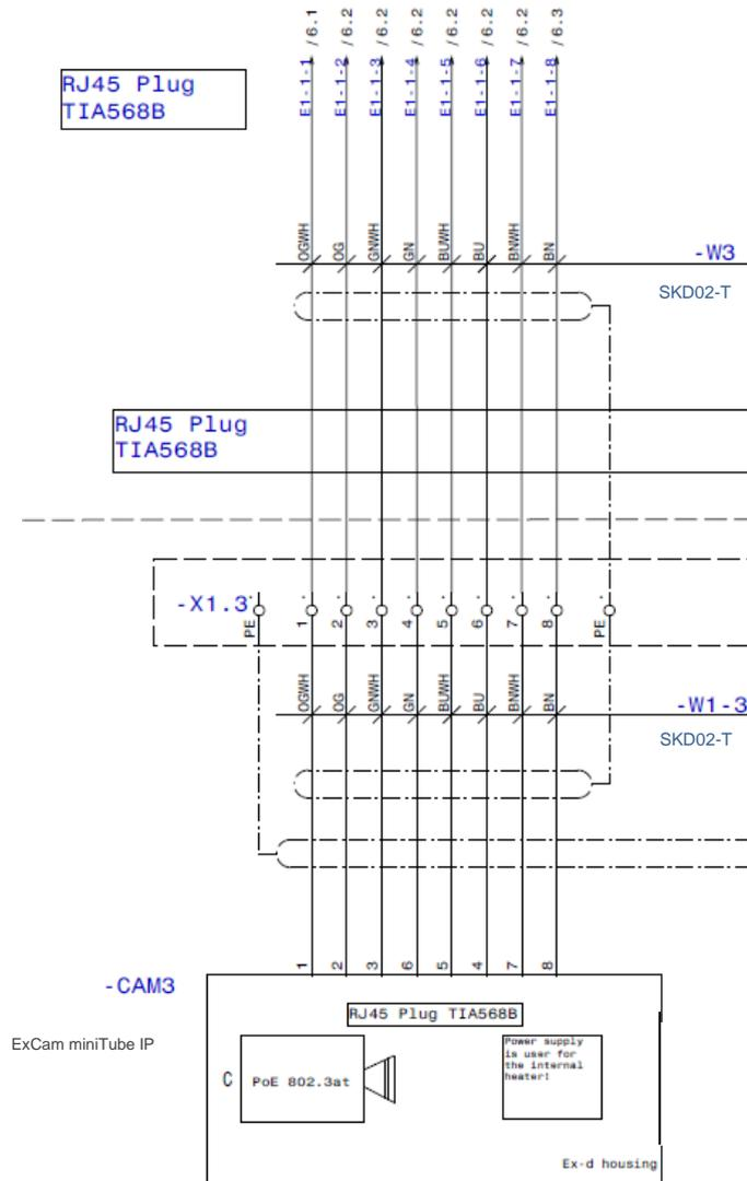
Figure 5-6 Sample circuit of terminal box ExTB-2
