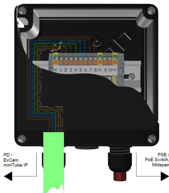
Figure 5.7 – Connection to the terminal box
