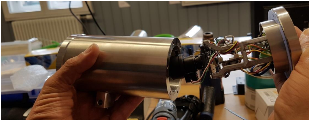
Figure 5.3 – removing the camera
